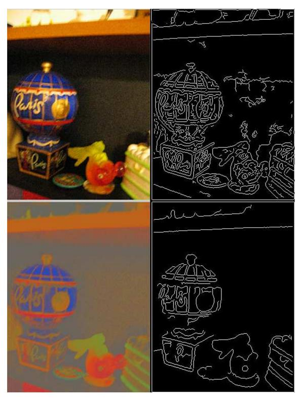
**Fig. 11.** Color correction for shadow contour removal I. Upper left is the original image. Upper right shows the edges of the original image. Lower left is the color corrected image and lower right shows the associated edges. The color correction simplifies the contour map by removing shadow contours. It also makes the contour map less dependent on illumination, which would be useful in such applications as object recognition.
